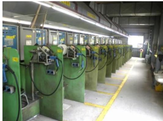
Fig. 9 Training Equipment for Training in IMB. Wall, Hanger, and Some of Equipment was Constructed by Trainers. In some regions, Japan Foundation donates welders and other devices for training.
