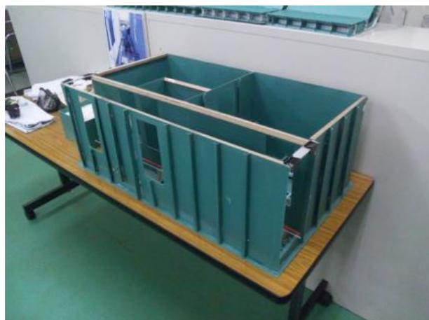
**Fig. 6 Paper-crafted Model of Bock (a part of ships' hull). This leads trainee to understand structure of hull, piping, and other instruments.**
